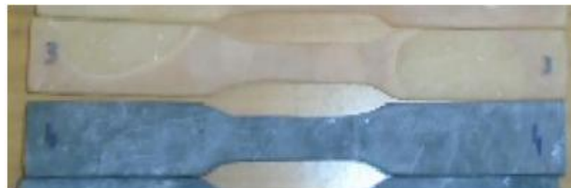
Figure 3.1: Tensile Test Specimen With Additives Calcium Silicate Or Silicon Carbide.
