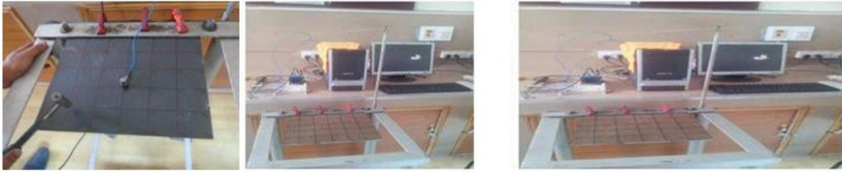
Figure 3.2.1: Modal Analysis Specimen Placed Testing
